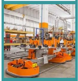
Fori Automation Inc. is modernizing the assembly line of a large U.S. automobile plant with rail guided carts with Siemens. The use of the SIMATIC S7-1200 controller is part of a fail-safe, automatic conveying and handling system. Watch the video to learn how Fori Automation was able to reduce time and labor required by 25 percent.
