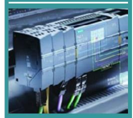
SIMATIC S7-1200 Basic Controllers are the ideal choice when it comes to flexibly and efficiently performing automation tasks in the lower to medium performance range. They feature a comprehensive range of technological functions and integrated IOs as well as an especially compact and space-saving design. Thanks to extensive expansion options, SIMAT-IC S7-1200 can be perfectly tailored to the specific automation task. SIEMENS Ingenuity for life
