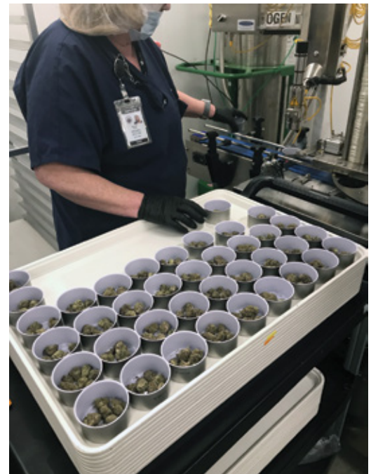
Aluminum cans for flower products are manually filled before being fed to an N2 nitrogen dosing and can seaming system.
