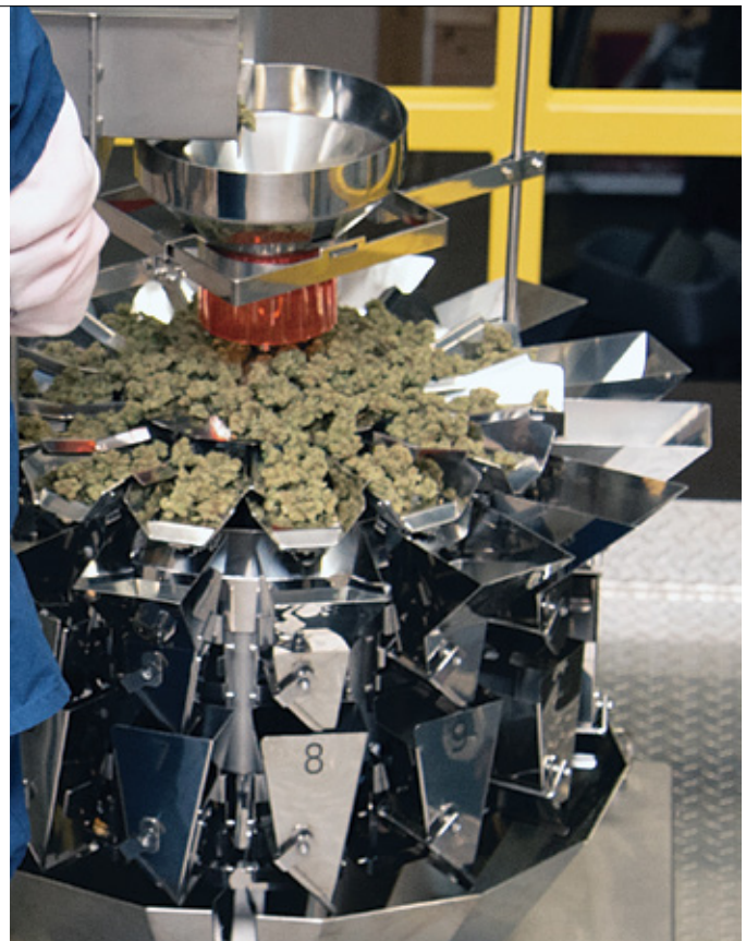
The multi-head Ishida weigher accurately weighs buds before dropping them to the pouch filler.
