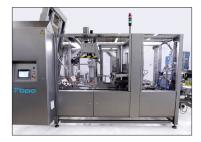
The Wraparound 100 is a highly flexible, modern, servo controlled horizontal case packer. It distinguishes itself with its unique Catamaran construction style, and is able to produce different case styles, offering you a large size range.
