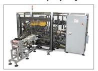
The HD-RSP is a compact cartoner that utilizes AFA or Fanuc Delta 3 robots to pick, orient, and collate product from upstream equipment. Applications include sachets, pouches, bags, bars, and stick packs.
