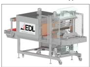
Designed for applications with lower throughput requirements, semi-automatic wrapper relies on operator to load and activate each wrapping sequence.
