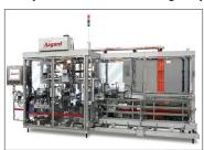
The Acclaim® Knock Down Case Packer can handle a wide range of products, including thermoformed trays, cups, and cartons. It orients the products for your desired case pattern by either tipping or not tipping the collated products via changeover.
