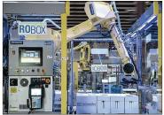
The 3rd gen. Robox is a modular and economical palletizer offered in over 20 pre-configured floor plans. With its compact footprint, it easily adapts to changing layouts and utilizes OptiStak, to set new or adjust pallet patterns directly from the HMI.
