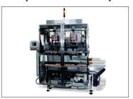
The HS Carton Erector / Tray Erector uses a 'direct placement' method of feeding the carton blanks into the forming tool, for an easy setup using factory-set tooling. The machine erects cartons and trays using a conventional four corner lock system or hot melt glue.
