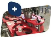
Retrofit existing change parts to quick change or add a new bottle size with replacement parts. We provide stars and guides for most machine manufacturers. O3 Container Handling Machinery
