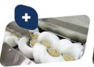
Meter, index, group, turn, twist, feed, combine and divide containers for a variety of your packaging applications. Each timing screw drive unit, combiner, and divider is designed to help increase your throughput.
